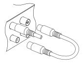
Whatever sort of connection you have between the digital receiver and the television, you need to connect the digital receiver to your television antenna so that it can receive digital television services.
